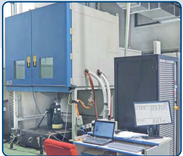
Digatron test bench for electric vehicle batteries
